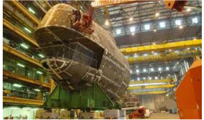
A Submarine under Construction in the Hall
