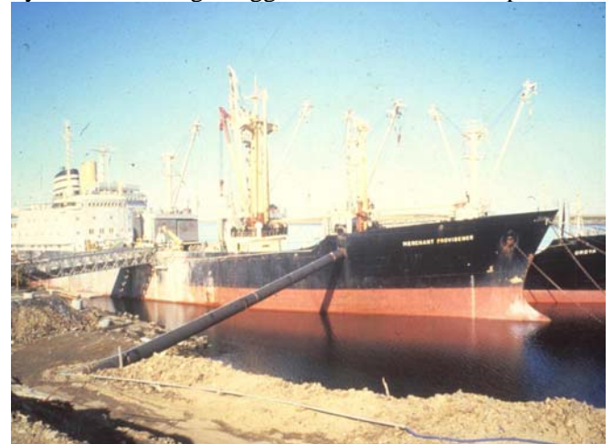
MV Merchant Providence secured as a Jetty Head
