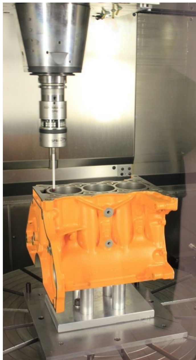
A probe being used to check the internal co-ordinates of a cylinder in an engine block.
